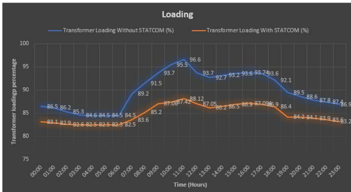
Figure 4.11. Analyses of hourly transformer loading
