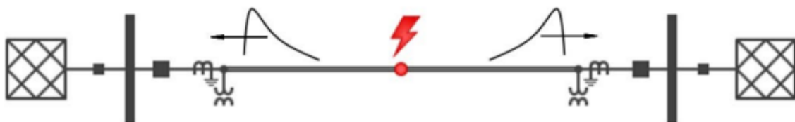
Fig. 3.1. Simple principle of traveling wave propagation
