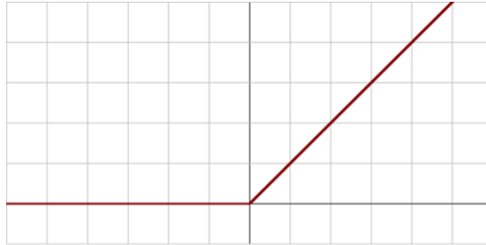
Figure 10. Rectified Linear Unit Activation Function ( https://en.wikipedia.org/wiki/Activation_function )
